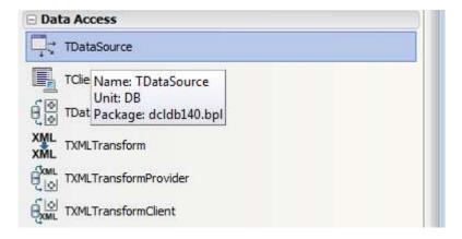
12. Hit the F11 key to bring forward the Object Inspector. In the Object Inspector, click on the DataSet property and change its value to **EDBTable1**.
